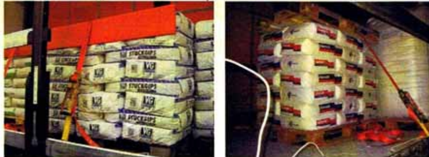
Alternative securing of a load unit by a pallet placed on top.
